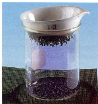
Iodine crystals at the bottom of the beaker vaporize into a gas, which then redeposits under the evaporating dish and becomes solid again.
