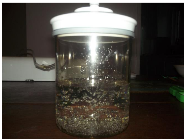
Air has been removed from the container. Notice that there are now more bubbles rising to the surface.
