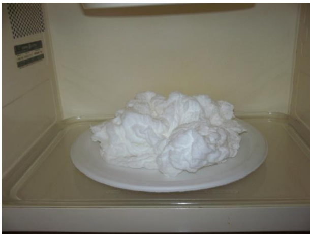
A bar of Ivory soap after being heated in a microwave. The heating causes the pockets of air in the soap to expand. This demonstrates the concept of Charles's law.
