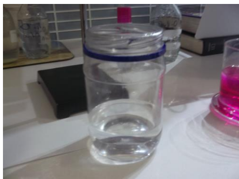
Acetic acid solution before titration. The solution contains phenolphthalein.
